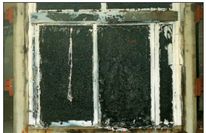
Fire side of sliding door after fire test made at SINTEF, Norway
