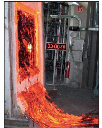
Object testing for fire resistance class 3 hours (EI 180 equiv) acc UL on the way to the "hose stream" part of the test
