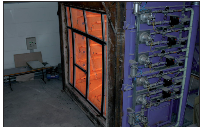
Fire test of a double door with top and side lights for fire resistance class E 60
