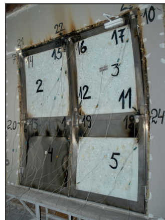
Fire test of a standard door with, e.g. screw-on hinges, wide mid bar, etc.
