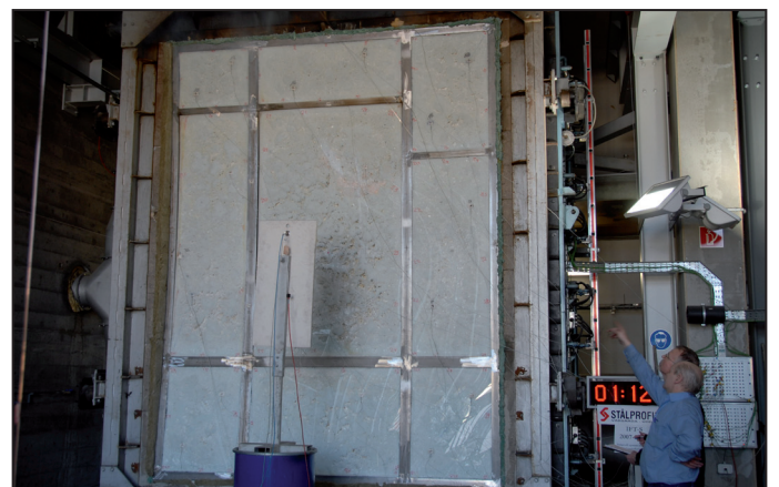
Fire test of 4 m-high wall section with "free edge" for fire resistance EI 60 as per EN
