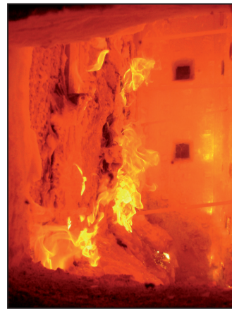
Furnace side of a section after approx 90 minutes during an EI 120 fire test
