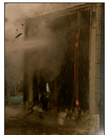
"Hose stream" test of door section for 90 min (EI 90 equiv) fire test in the US.
